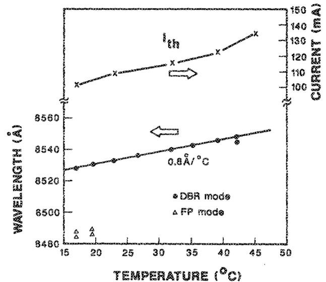
FIG. 4. Variation of threshold current  $I_{\text{th}}$  and lasing wavelength with temperature. The  $I_{\text{th}}$  followed a straight line except for a dip at around 35 °C, corresponding to the coincidence of the gain peak and the Bragg wavelength. Single wavelength operation is observed from 20 to 40 °C.
