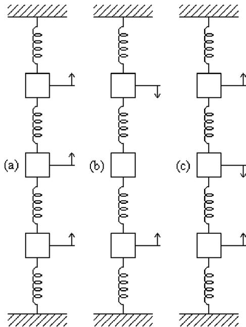
Fig. 3. Modes of vibration for a system of coupled oscillators with three masses and four springs. (a) Normal mode with the lowest frequency. The motion of the three masses is in phase. (b) Normal mode with intermediate frequency. The central mass is at rest and the motion of the other masses is out of phase. (c) Highest frequency normal mode. The motion of the outer masses is in phase while the motion of center mass is out of phase with the others.
