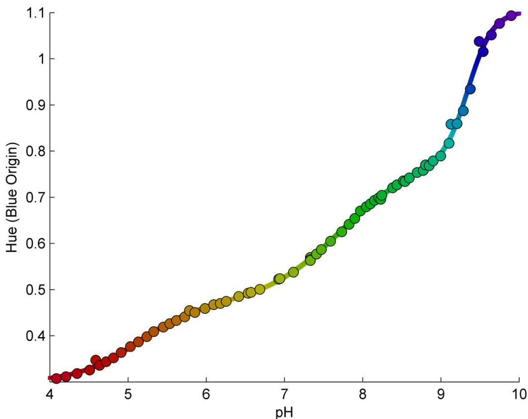
Figure 6: Hue-pH Calibration Curve for Universal Indicator
