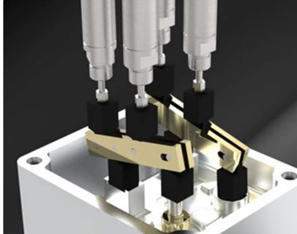
Figure 15: Model of Rocker Valve Actuation System
