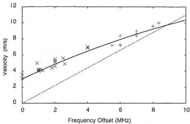
Fig. 3. Measured velocity of atoms leaving the funnel as a function of the frequency offset  $\Delta f$  of the horizontal lasers. The  $\times$  symbols (+ symbols) correspond to a mean laser detuning of  $2\Gamma$  ( $3\Gamma$ ) from resonance. The dotted line is the expected velocity of a moving molasses. The solid curve represents a more detailed model that includes an axial magnetic field (4G) and the finite damping time (1.2 ms) of the atoms in the molasses.
